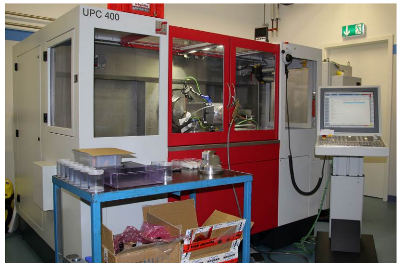
Fig. 1 and 2: Ultra-precision milling machines to produce high-precision surfaces
