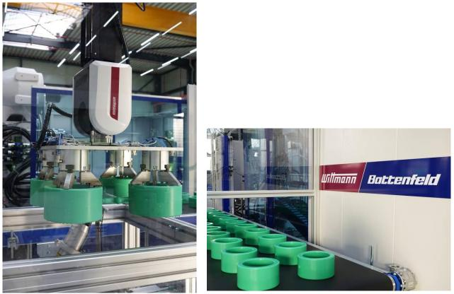
Fig. 5a+5b: Parts removal and depositing with WITTMANN W843 pro robot (photos: aquatherm)
