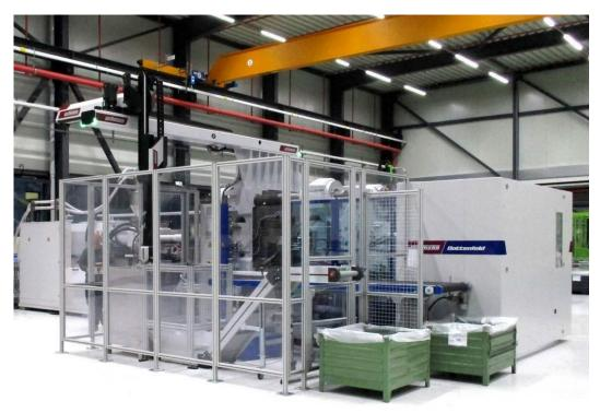
Fig. 4: MacroPower 1000/16800 with customized automation (photo: aquatherm)
