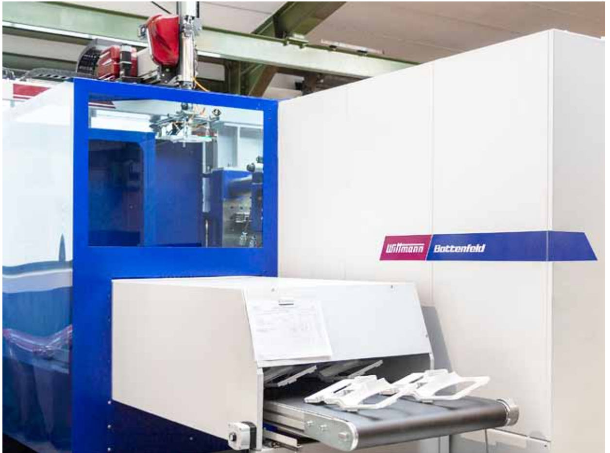
Production of a housing component for a beverage dispenser with SmartPower 300/1330 with Insider cell.
